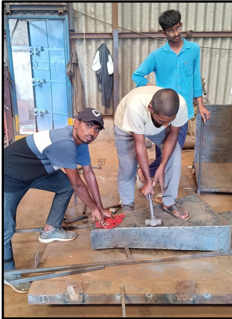
Fig 3.22. Fabricating the bucket 2
