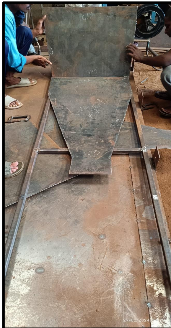
Fig 3.19. Fabricating the Bucket frame
