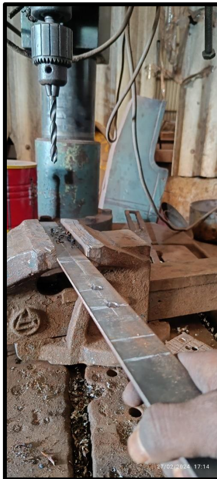
Fig 3.24. Drilling the holes for Hooks
