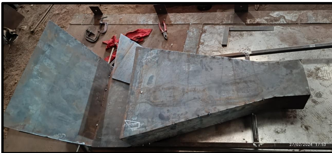
Fig 3.23. Fabricating the bucket 3
