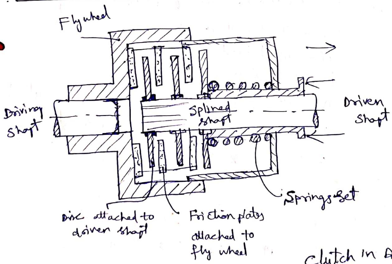
clutch in disengaged position.
