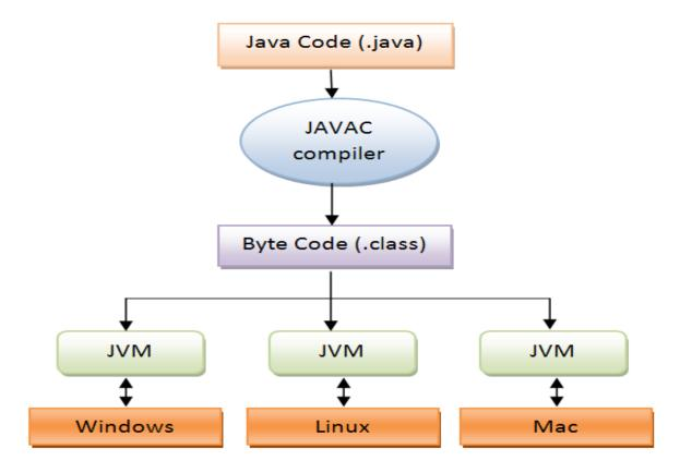
Java's Magic: The Bytecode output of a Java compiler is not executable code. Rather, it is bytecode. Bytecode is a highly optimized set of instructions designed to be executed by the Java run-time system, which is called the Java Virtual Machine (JVM).
