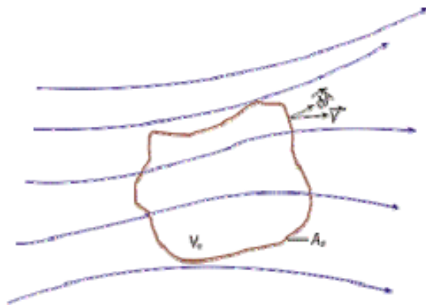
FIG 4.1 Finite control volume fixed in space with the fluid moving through it
