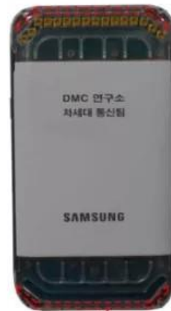
16-antenna arrays at the top and bottom of a prototype Samsung phone CREDIT: SAMSUNG
