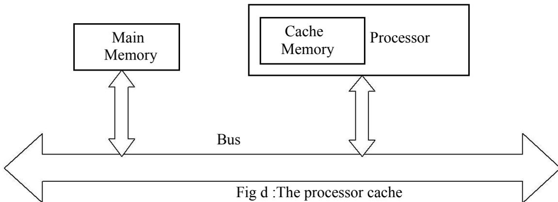
The pertinent parts of the fig. c is repeated in fig. d which includes the cache memory as part of the processor unit.
